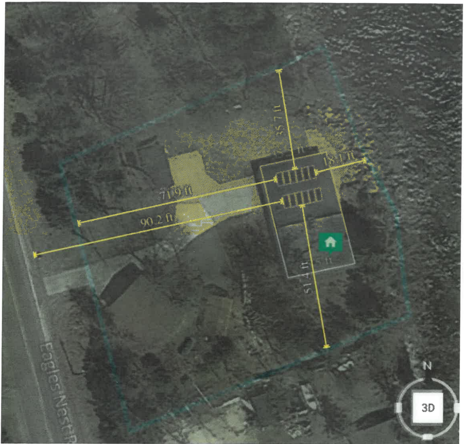
Roof Mounted PV Array Site Plan
